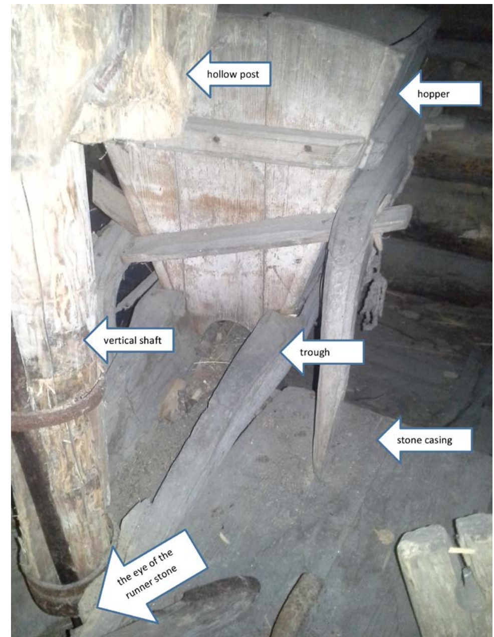
Figure 6.3. The ancient hopper and trough were designed to lead the grains into the eye of the runner stone. Photograph by Gustaf Lindroos.
