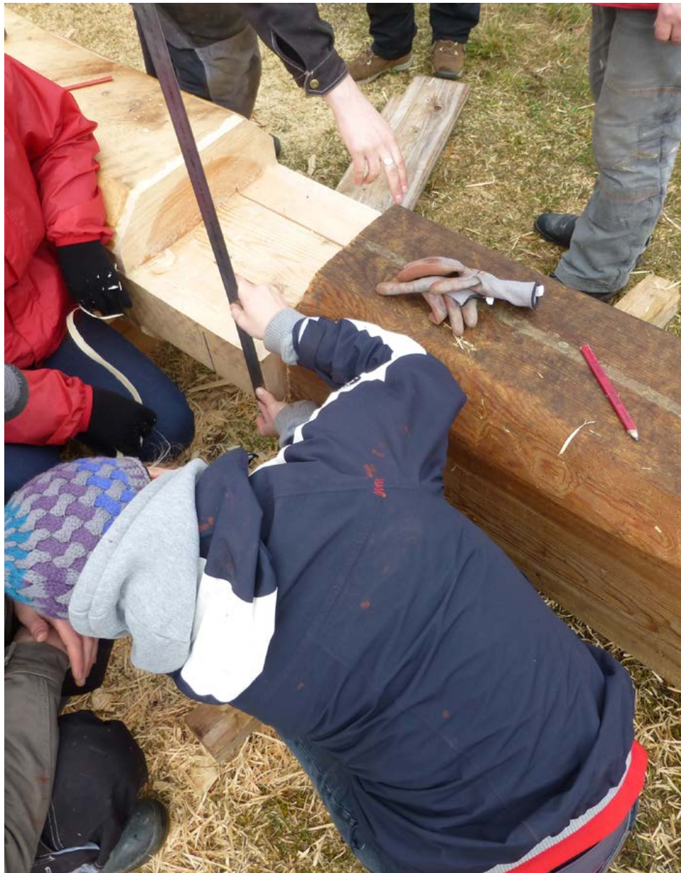
Figure 1.7. The making of the open mortise and tenon joint took a lot of planning and measuring, sawing, planing and fitting before the pieces matched perfectly. Photograph by Kirsti Horn.
