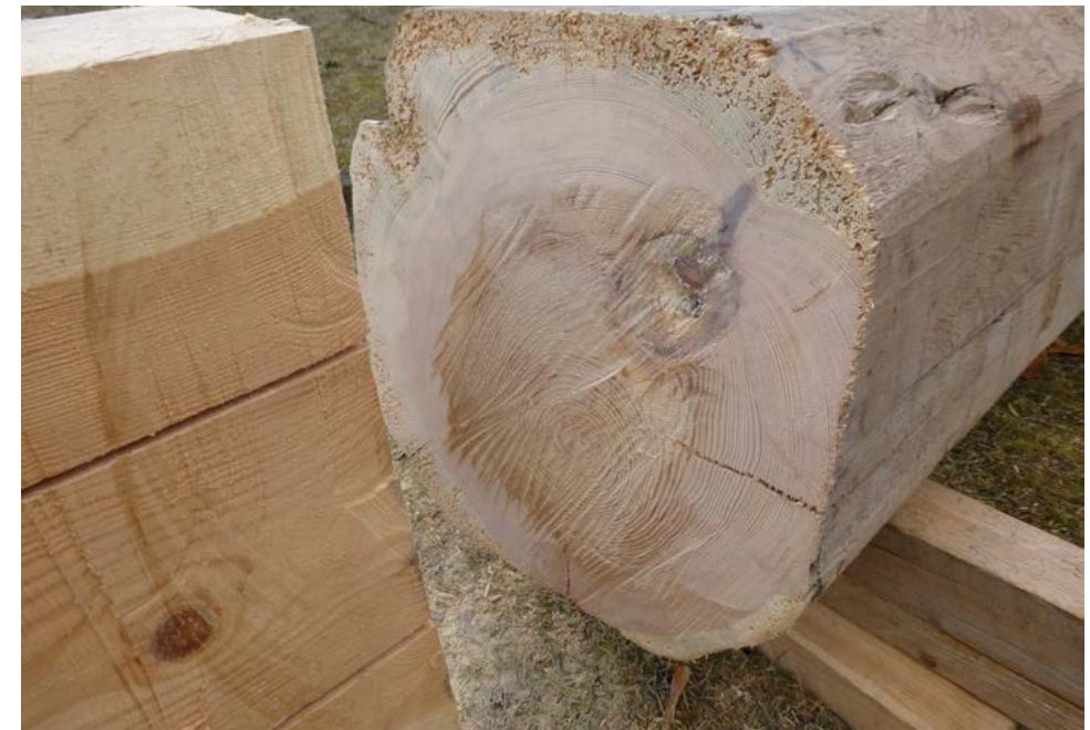
Figure 1.6. The section of the original wind shaft on the right reveals the destruction by insects. Photograph by Kirsti Horn.
