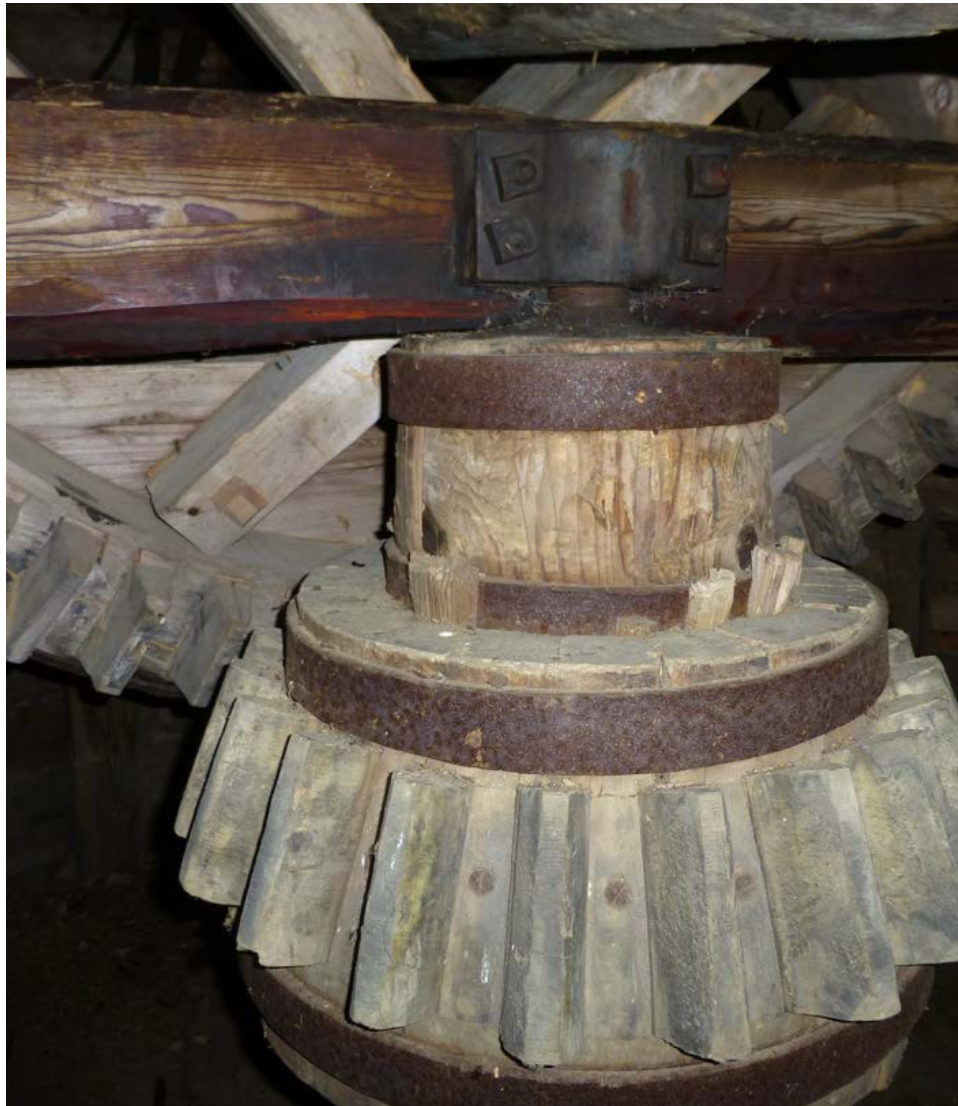
Figure 7.7. The bevel wallover on top of the upright shaft is made of sections that could be replaced when they wore out. The brake wheel in the background is unfortunately not properly attached to the wind shaft . Oripää mill, Seurasaari, Helsinki. Photograph by Kirsti Horn.
