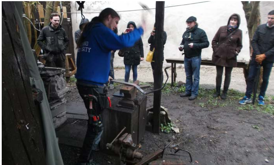
Figure 1.25. Visiting students admire John Friederich working in his forge in Visby. The skillful smith is beating out the big clamp for the joint between old and new parts of the wind shaft . Photograph by Kenneth Eriksson.
