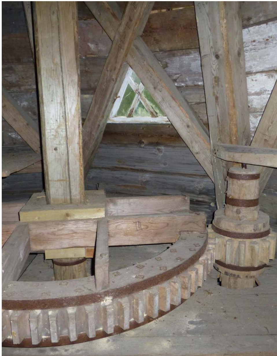
Figure 7.3. On second floor the pinion on top of the shaft turned a second upright shaft via a wooden clasp arm spur wheel. Oripää mill, Seurasaari, Helsinki. Photograph by Kirsti Horn.
