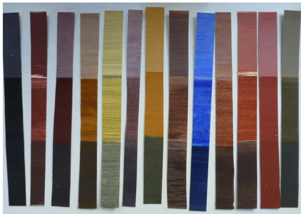
Figure 2.3. Experiments from the paint studio. Hues with various earth pigments and linseed oil: from left Kassel brown, Falun red, Terra di Siena, Terra, bright green earth, Caput Mortum, Ochre, burned Umbra, Ultramarine, burnt green earth, Terra di Pozzuoli, English red and burned Umbra. Photograph by Kirsti Horn.
