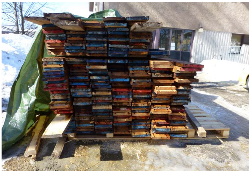
Figure P5. Everything ready for the intensive course together with Estonian and Swedish students: tarred roofing planks were piled in the open to avoid cracking. Photograph by Kirsti Horn.
