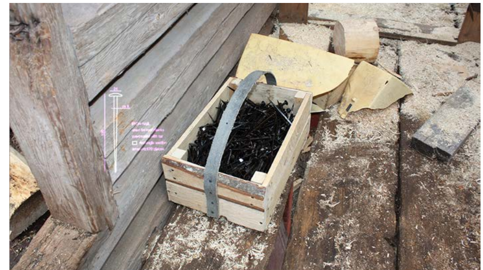
Figure 1.2. Siim Otsa, the Estonian black smith who made the nails for the roof, delivered them in a nice box. Photograph by Sille Sombri.
