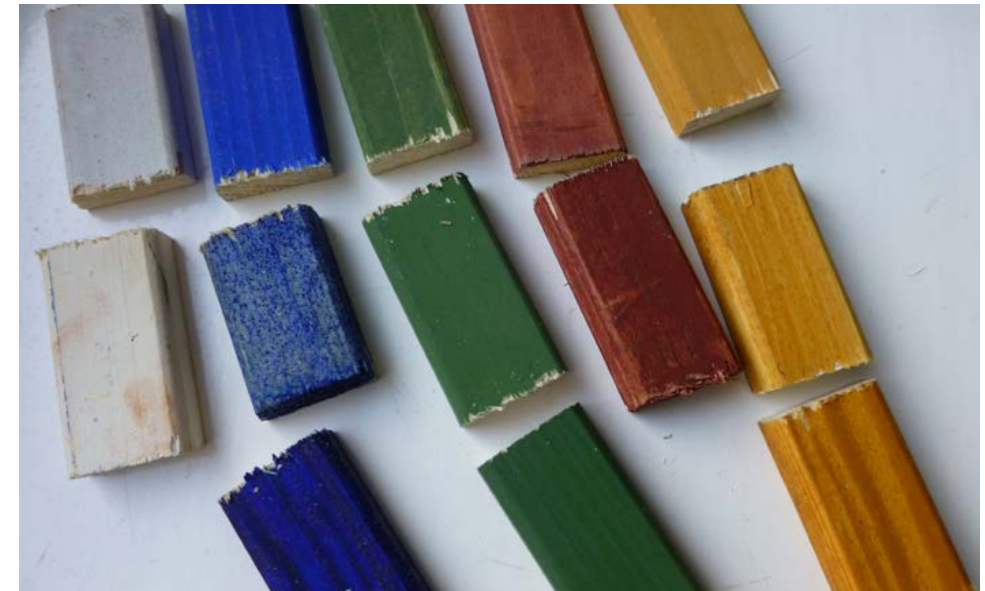
Figure 2.2. Experiments from the paint studio. Some of the samples of different pigments and binders: milk-cement in top row, petroleum in the middle, linseed oil at the bottom. Photograph by Kirsti Horn.
