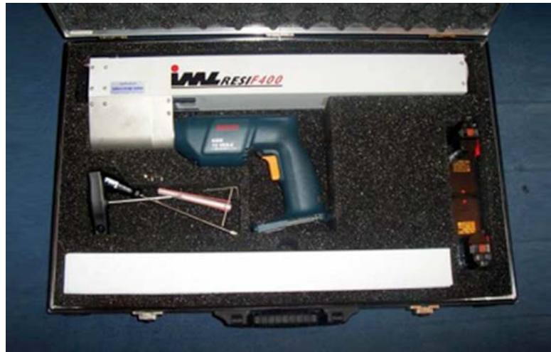
Figure 3.13. Micro drilling apparatus.
