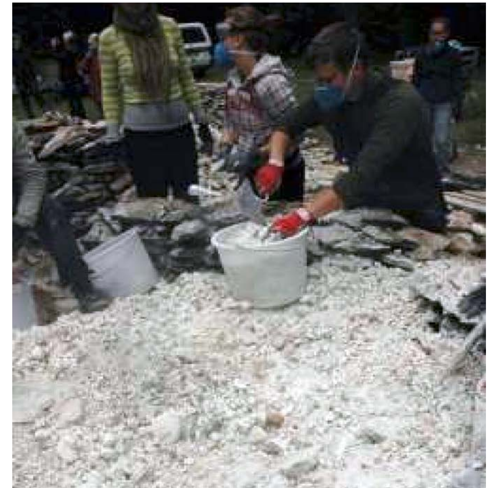
Figure 6. Emptying the lime kiln and sorting out the lime.
