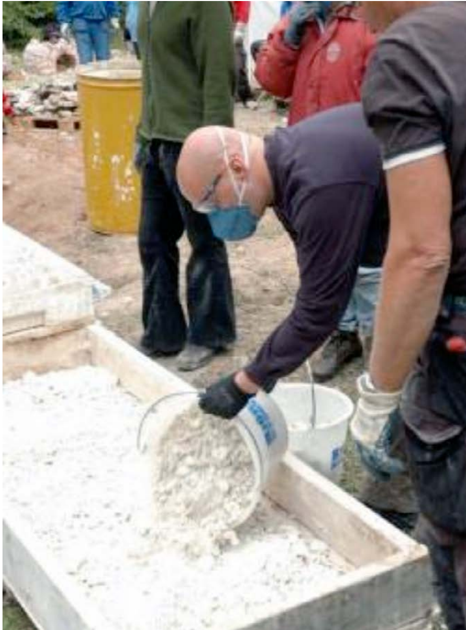
Figure 7. Sorting out the completely burned lime stone.
