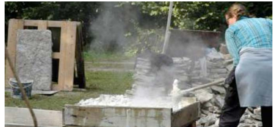
Figure 11. Wet slaking. Kristin Balksten in action.
